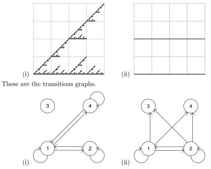
9. (b) To gennerate driven IFS (i), the time series exhibits all combinations of points in bins 1 and 2, and all combinations of points in bins 1 and 4. For (ii) no time series will generate the driven IFS: as soon as a data point enters bin 3 or bin 4, it can go nowhere.
