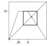
(a) The fixed points are circled. Both are unstable, because the slope of the graph of f is steeper than 1 at the fixed points.
