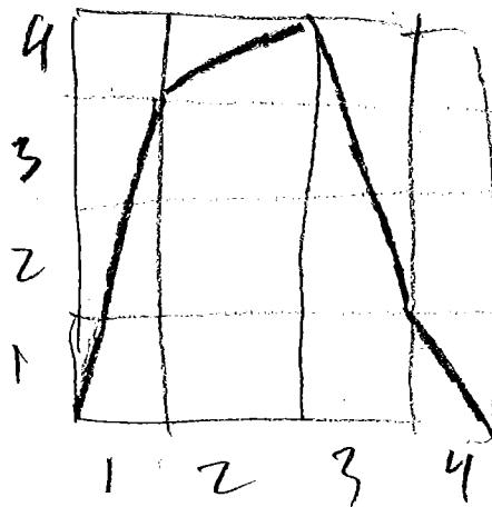
Above each bin on the x-axis, every bin on the y-axis that is entered, is crossed completely
