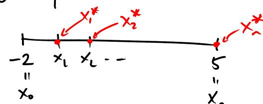
$$\begin{aligned} \text{Riemann sum. } \sum_{i=1}^n f(x_i^*) \cdot \Delta x &= \sum_{i=1}^n f\left(-2 + \frac{7i}{n}\right) \cdot \frac{7}{n} \\ &= \sum_{i=1}^n e^{2\left(-2 + \frac{7i}{n}\right) + 1} \cdot \frac{7}{n} \\ &= \frac{7}{n} \sum_{i=1}^n e^{-3 + \frac{14i}{n}} \end{aligned}$$
